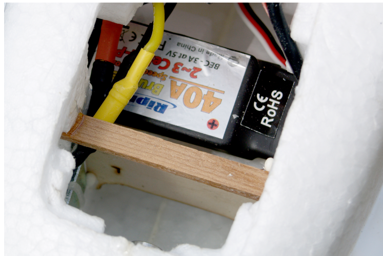
3 x 6 mm spruce cross-piece epoxied into the foam moulding
